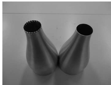
(a) Clean vs. Notched Nozzle Exit. (b) Sound pressure levels associated with a clean nozzle and a notched nozzle.
