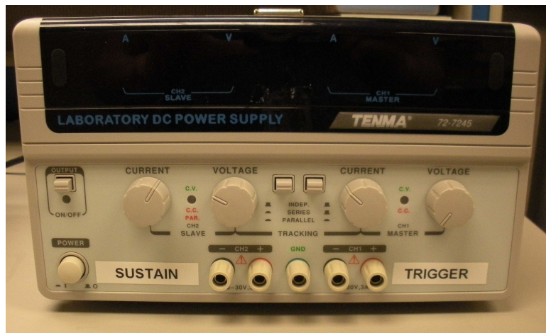
Figure 4.11: Photograph of the TENMA-72-7245 Dual Channel Bench DC Power Supply used to power the 600ET SparkJet circuit.
