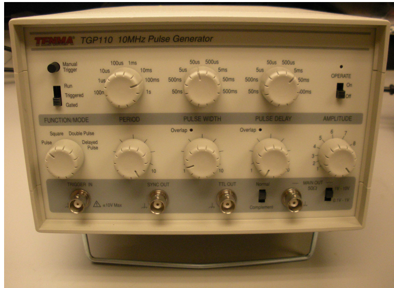
Figure 4.10: Photograph of the TENMA-72-6860 Pulse Generator used to trigger the 600ET SparkJet circuit.
