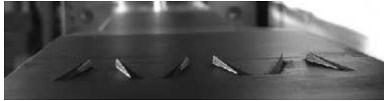
(a) Picture of vortex generators.
